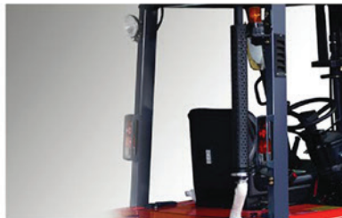
Upward Exhaust Pipe II
